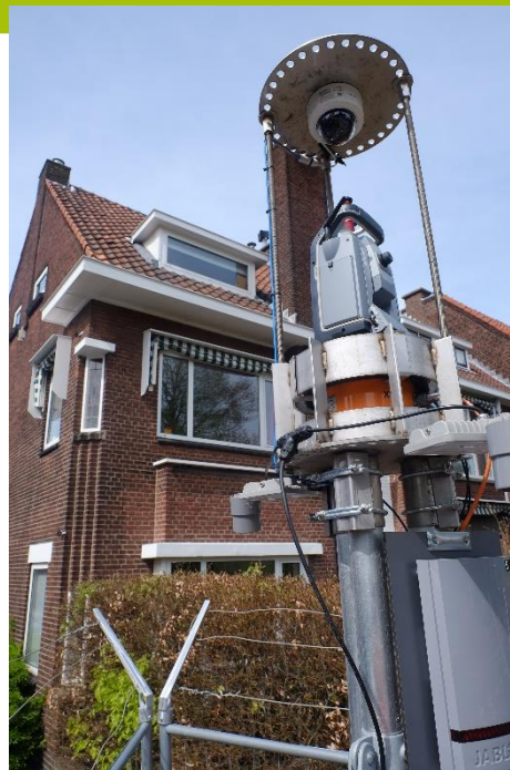
Robotic Total Station
